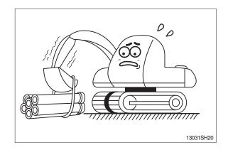
The operation on a slope is dangerous. Avoid operating the machine on a slope of over 10 degree.
